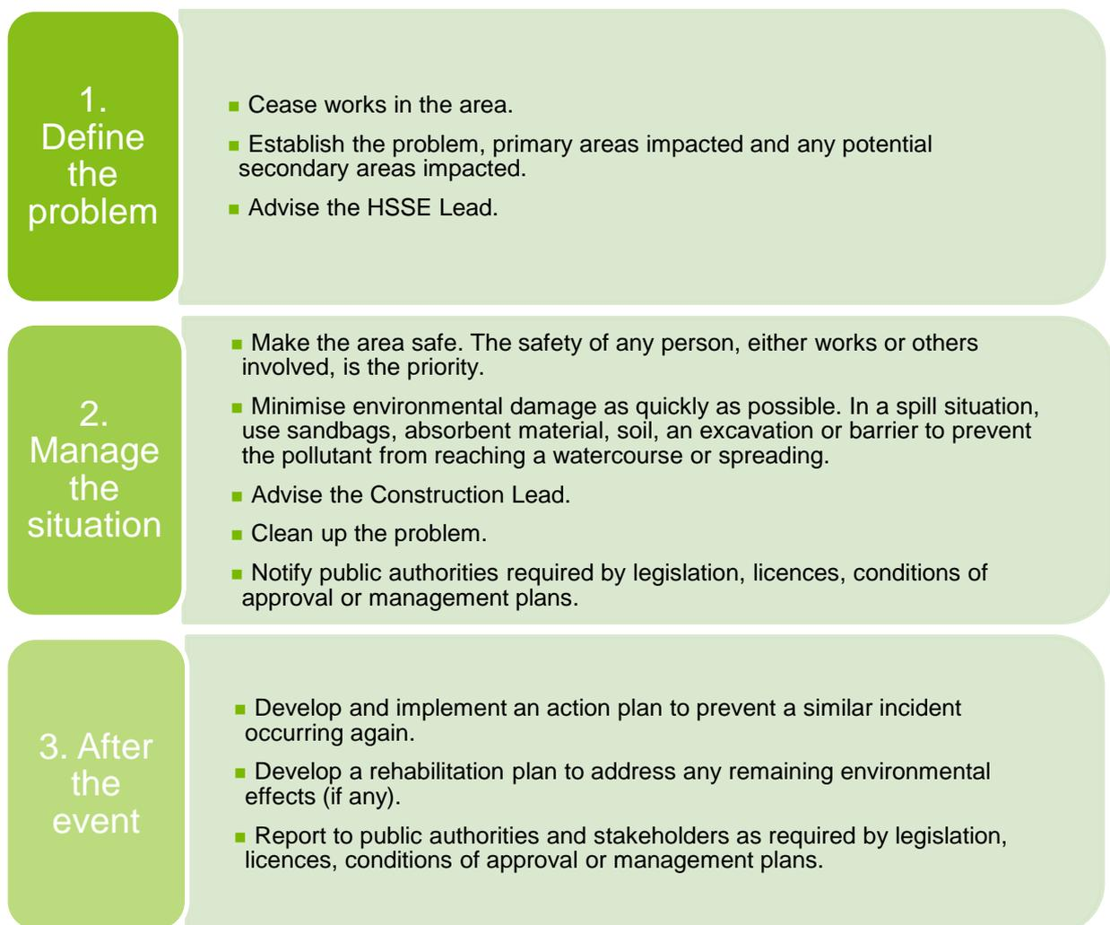
Figure 5-1 Emergency response procedure
