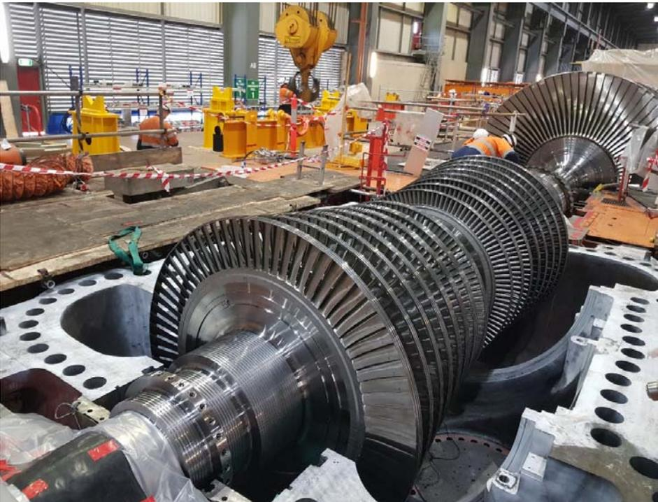
Test fitting the new Intermediate Pressure Turbine in its casing
