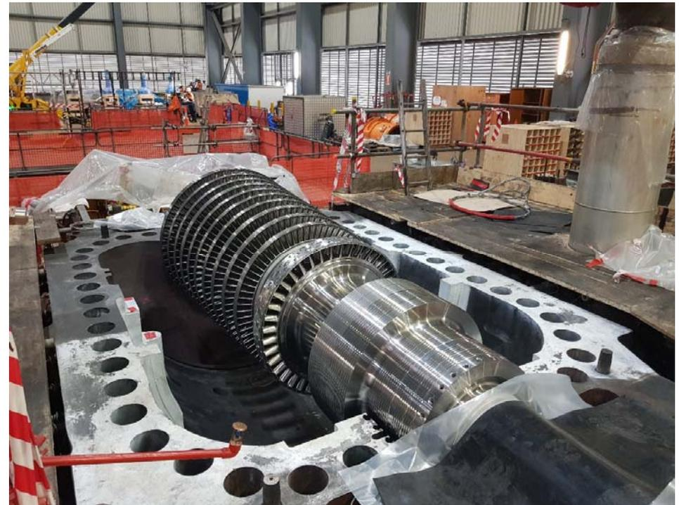
Test fitting the new High Pressure Turbine in its casing
