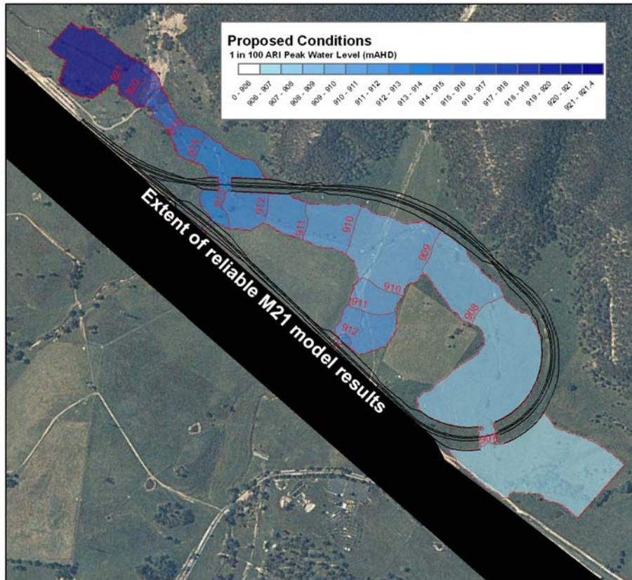
■ **Figure 5-2: Proposed conditions 100 year design flood peak water elevation.**
