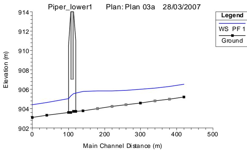
■ **Figure 4-8: Pipers creek outlet for proposed conditions.**
