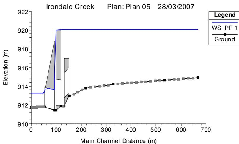
■ **Figure 4-4: Irondale Creek inlet for proposed conditions.**
