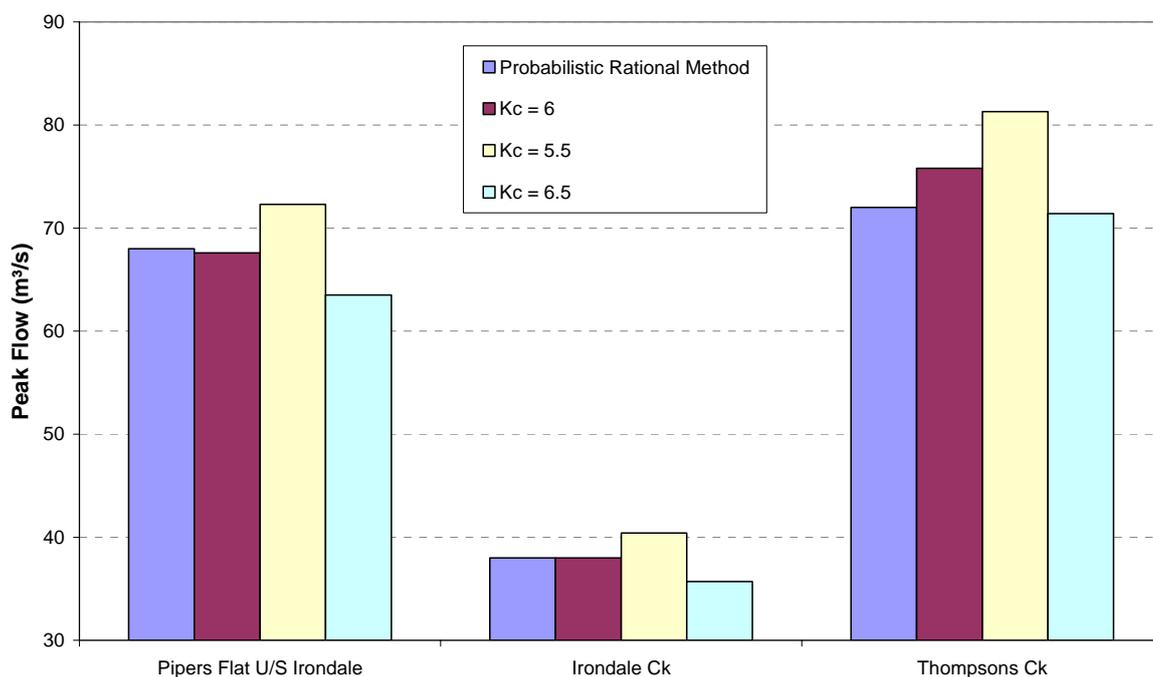
■ **Figure 3-1: Test of sensitivity of peak flow estimates to  $k_c$  with IL=6.0 and CL=2.5.**
