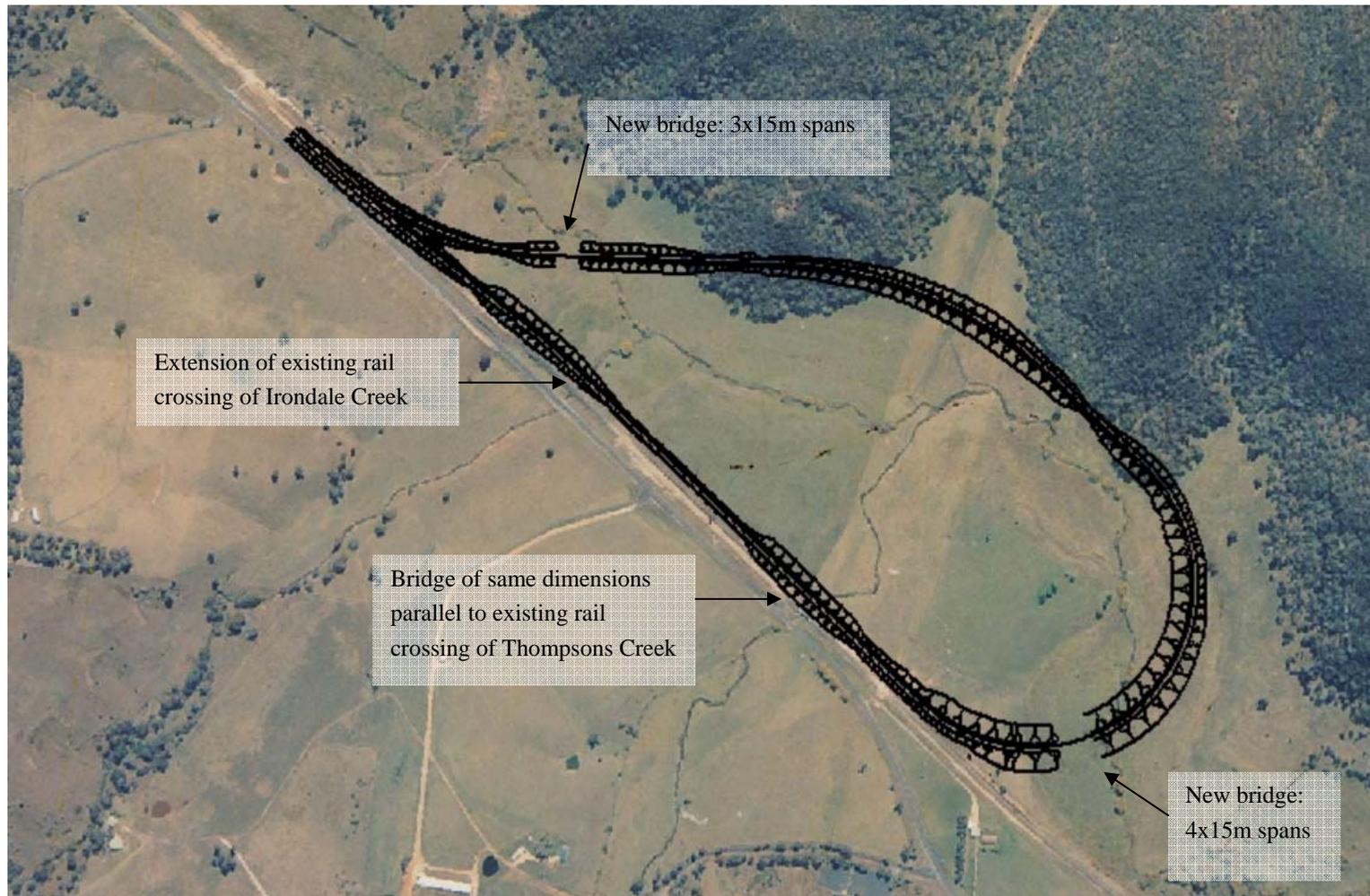
■ **Figure 2-3: Proposed design of loop and additional waterway crossings at Pipers Flat**
