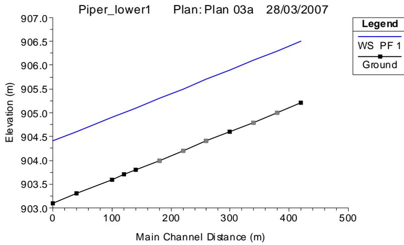
■ **Figure 4-7: Pipers Creek outlet for existing conditions.**
