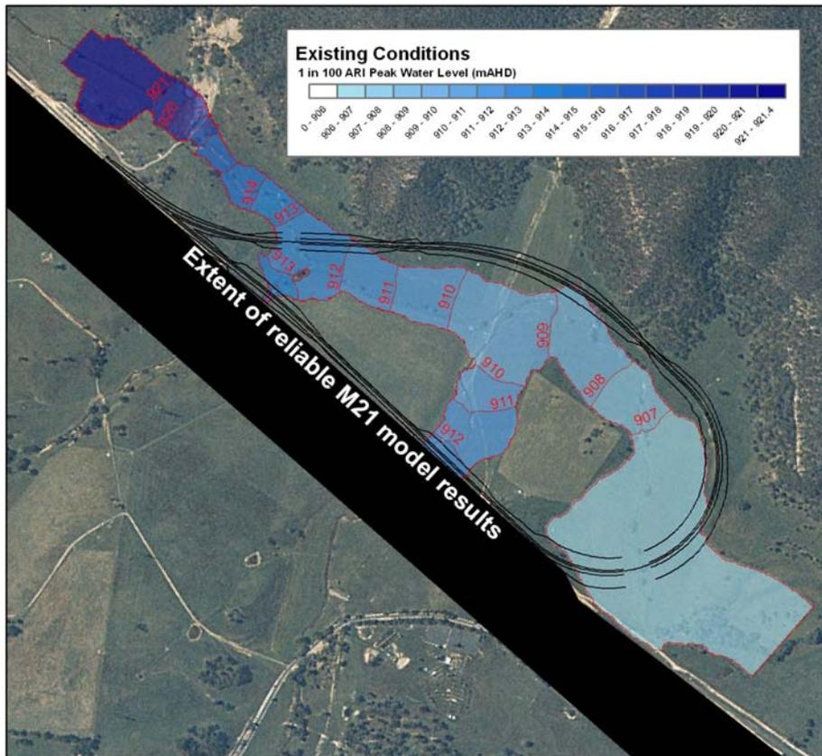
■ **Figure 5-1: Existing conditions 100 year design flood peak water elevation.**
