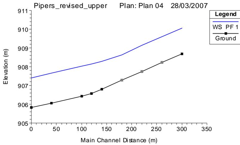
■ **Figure 4-5: Pipers Creek inlet for existing conditions.**
