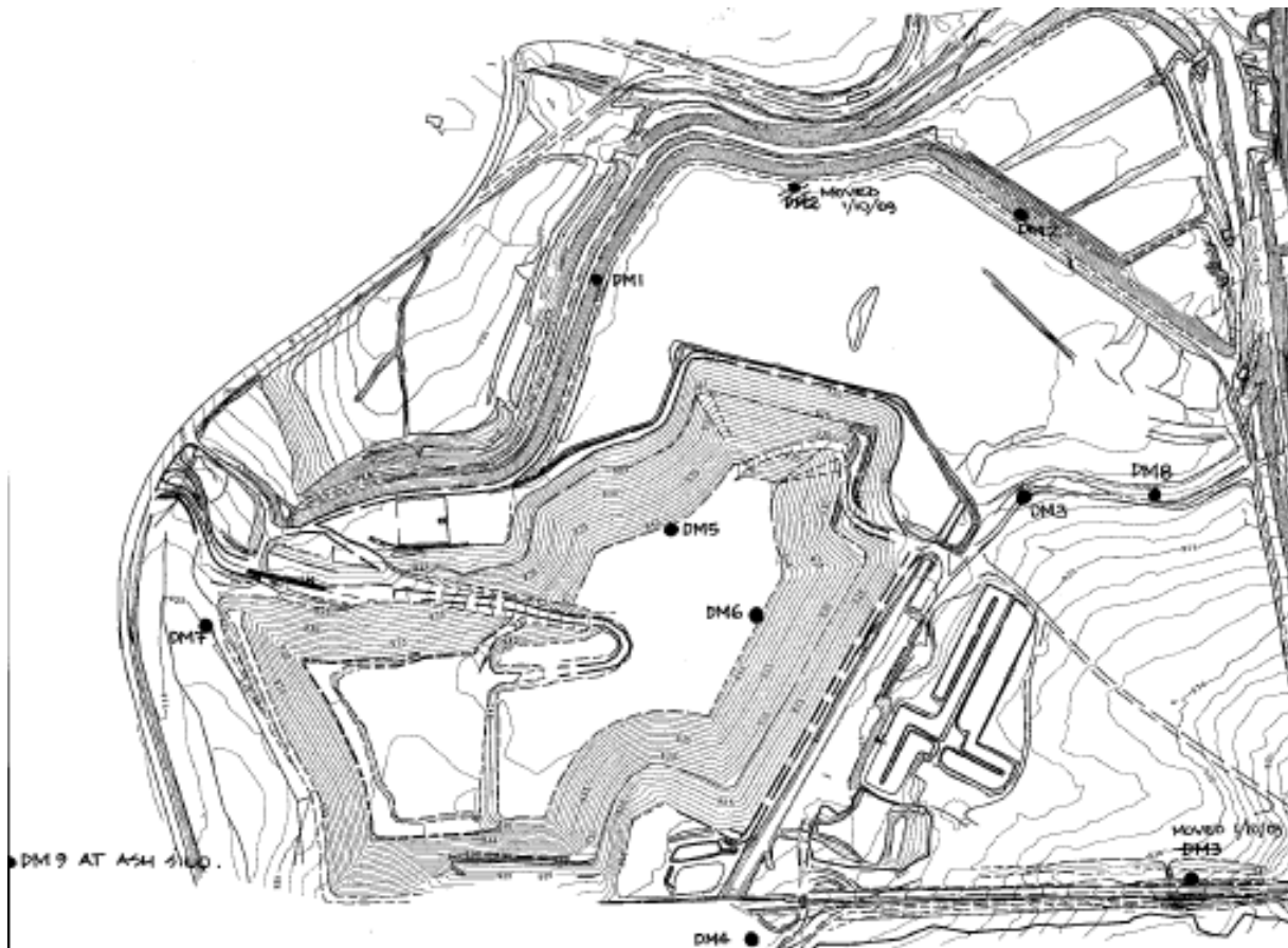
Figure 3: Location of dust gauges operated in and on the perimeter of KVAR2 operated by the site contractors. Note that DM9 is located at the ash silo about 1,500m to the south-west at Wallerawang Power Station.
