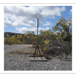
Plate 2: Dust deposition gauge 23 located near the **Lamberts North emplacement**
