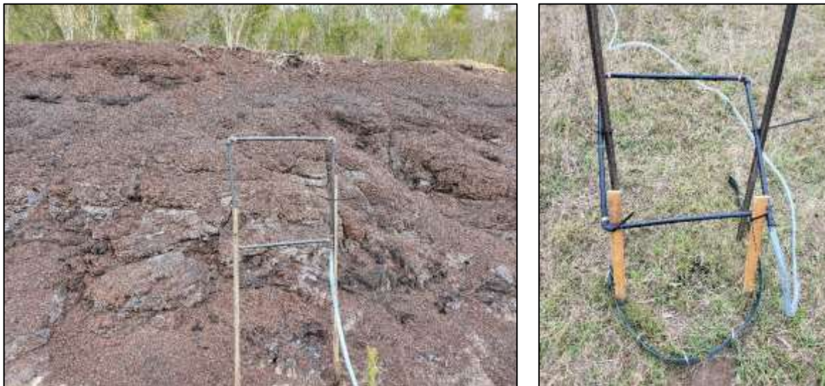
Figure 2-6: Wall washing experiments on weathered coal (left) and topsoil/overburden (right) showing spay headers manifold
