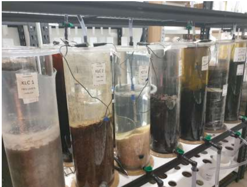
Figure 2-7: Kinetic leach column (KLC) tests for YCM at RGS Laboratory.
