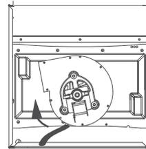
4. Reconnect flue fan extension using silicon to seal connection. Secure flue outlet to side panel using screws previously removed. Fit flue outlet cover to the original outlet hole.
