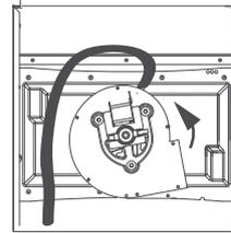
3. Turn combustion fan 180 degrees. locate fan feet in 4 round holes in flue pan twisting combustion fan towards burners to lock.
