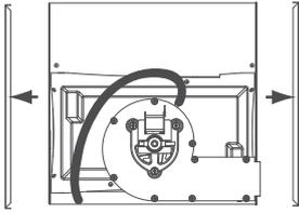
2. Twist combustion fan towards burners, lift fan up to separate from heater.
