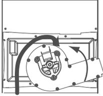
3. Turn combustion fan 180 degrees. locate fan feet in 4 round holes in flue pan twisting combustion fan towards burners to lock.
