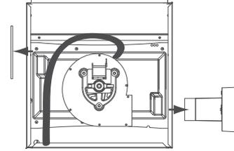
2. Twist combustion fan towards burners, lift fan up to separate from heater.
