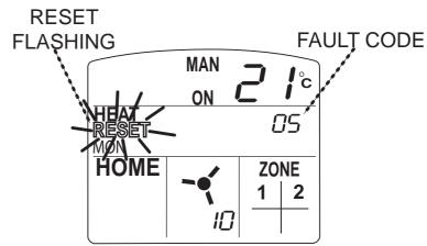
DISPLAY WITH FAULT DETECTED
