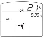
Fan-only display with zones 1, 2 and 3 on - single SCC with zones, or multiple SCC system.
