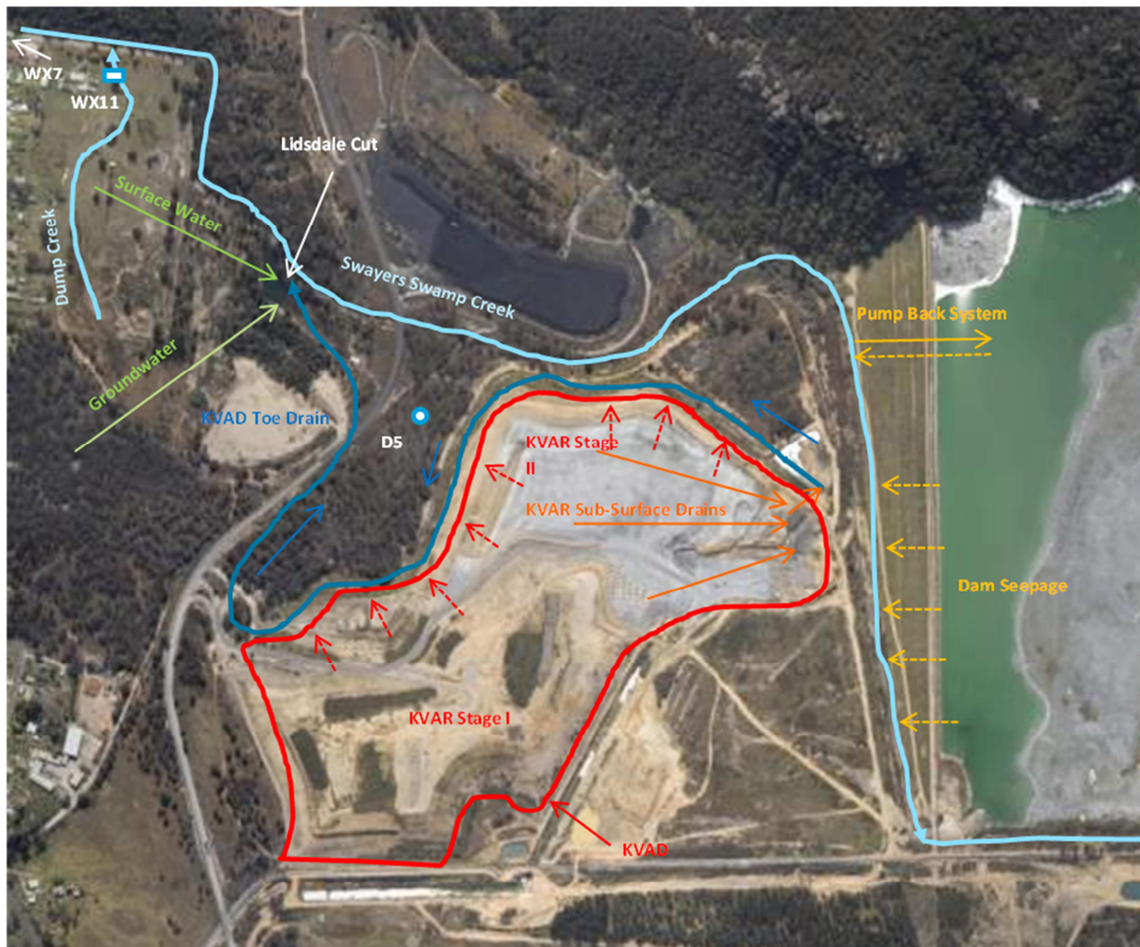
Plate 1. Schematic of Sawyers Swamp Creek Ash Dam and KVAD/R seepage flow paths to the KVAD toe drains and Lidsdale Cut
