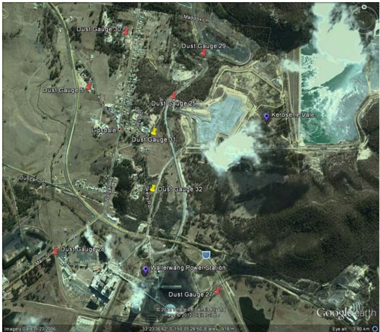
Figure 5 Dust Gauges located around KVAR (Google Earth, 2012)
