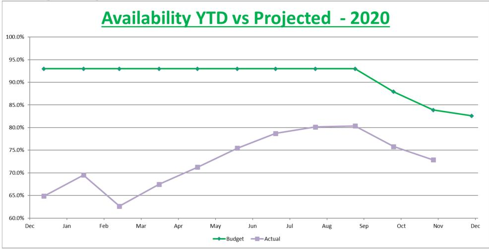
Negative Impact of Secondary Superheater failures was a significant poor start to the year.
