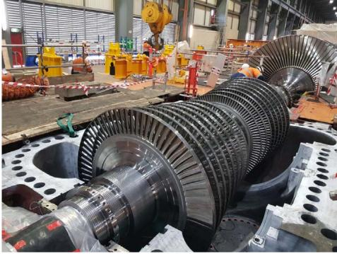
Test fitting the new Intermediate Pressure Turbine in its casing As the pressure decreases, the volume of steam increases, requ
