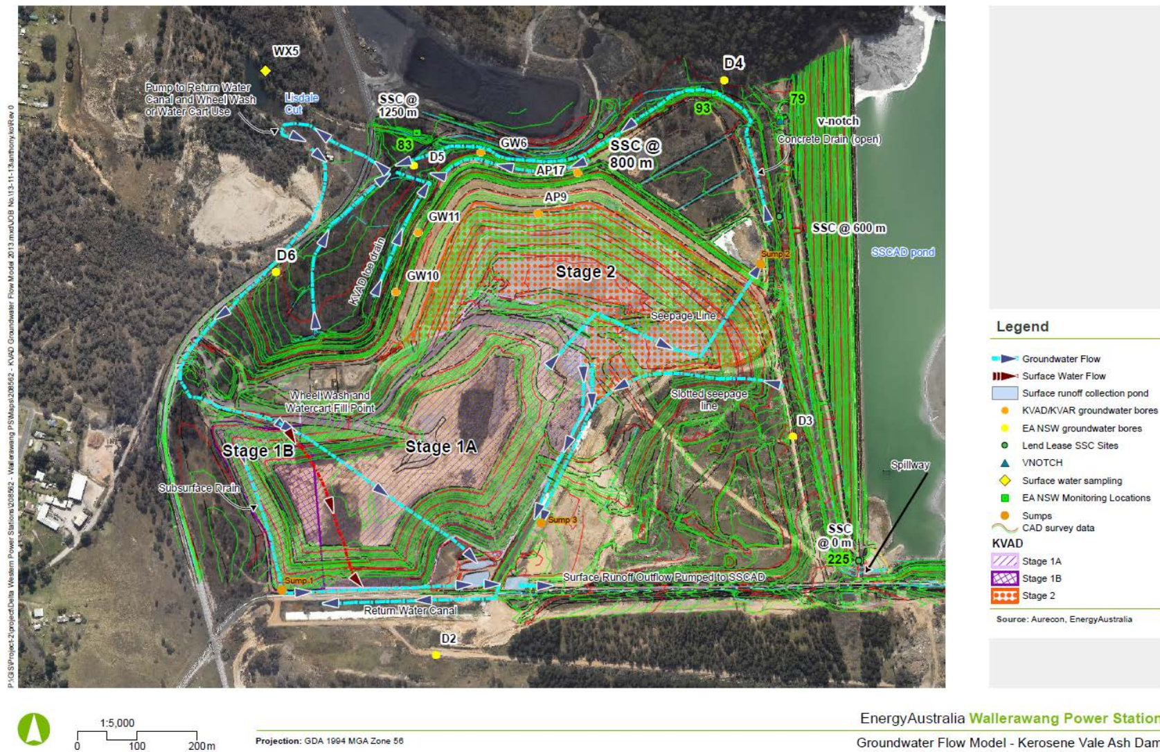
Figure 1: Schematic of Kerosene Vale Dry Ash Placement Area Seepage Diversion works
