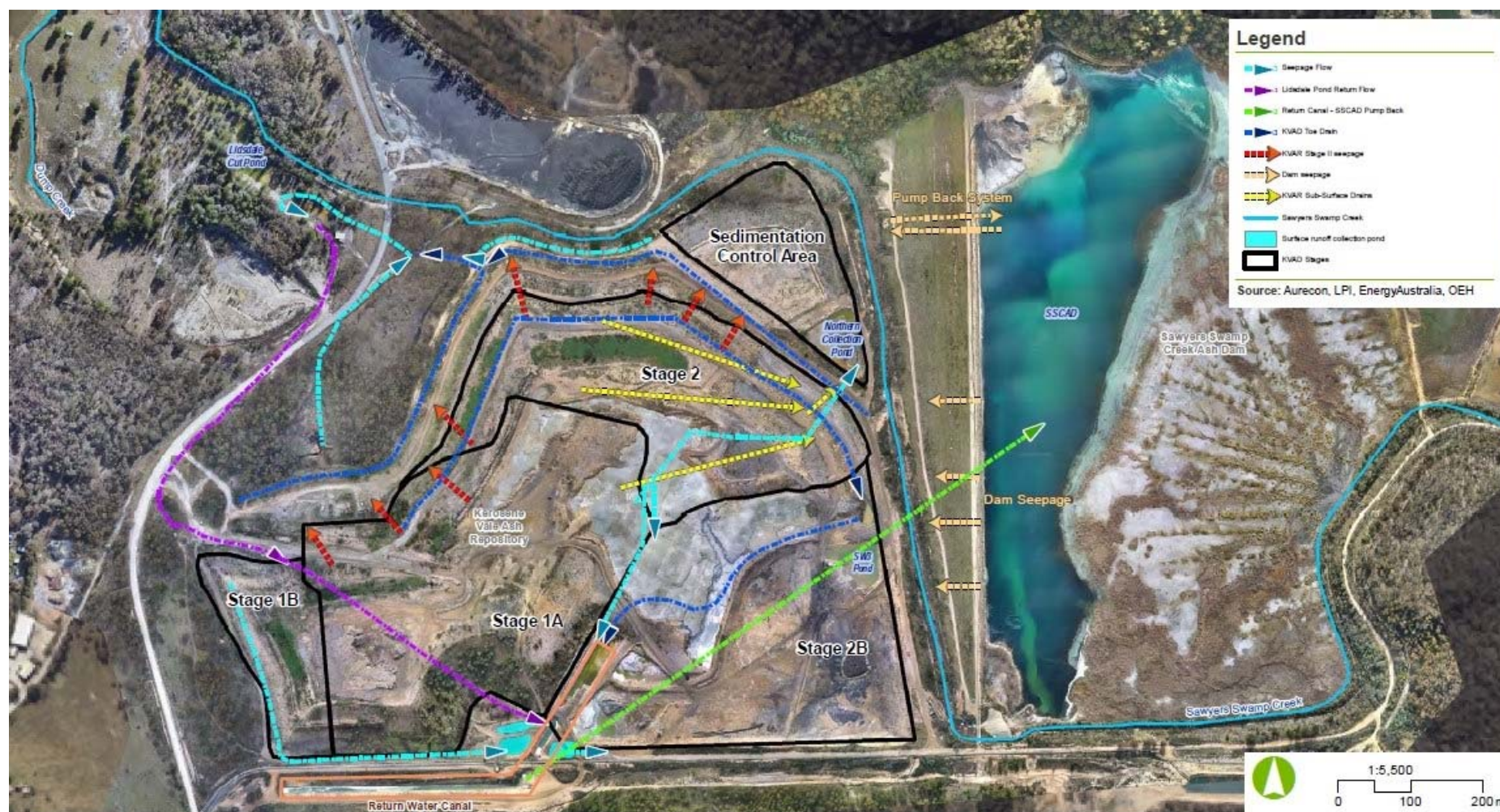
Figure 19: Existing site drainage system
